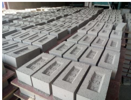
Figure 2. A brick sample made on the basis of a mixture of coal ash.
