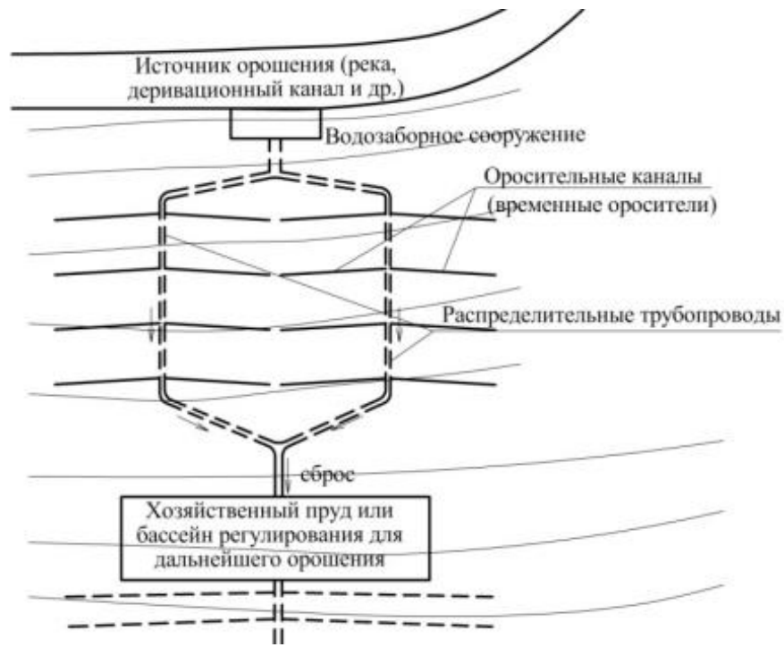
Figure 1 - Energy-saving pressureless design of irrigation system distribution pipes with ring network device
