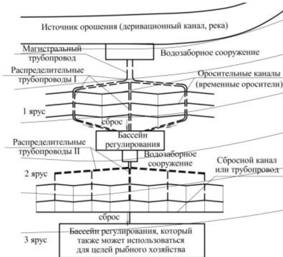
Figure 3 - Energy-saving non-pressurized design step irrigation system distribution pipes
